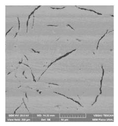
**Figure 1.** Micrograph of gray cast iron without biodiesel exposure. 2000X. Polished with alumina 10  $\mu$ m. Lamellar graphite with perlitic phase in the matrix.
