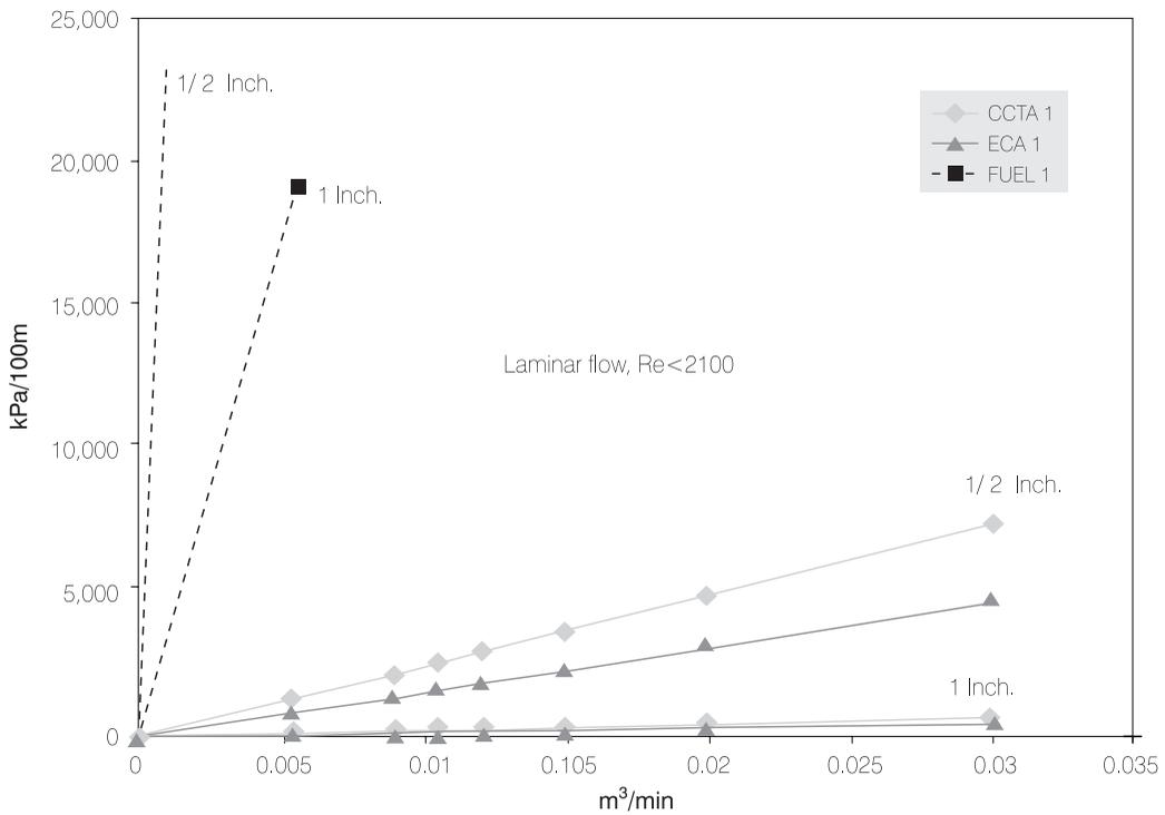
Figure 4b. CCTA mixture, pipeline transport simulation, 293 K
