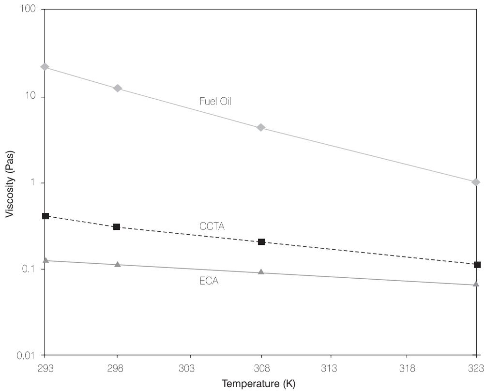
Figure 3b. Viscosity curve of fuels evaluated
