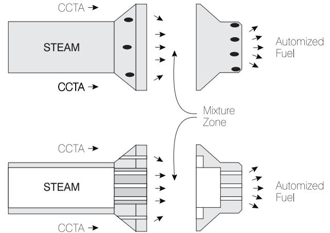
Figure 2. Type of nozzle configuration used in the combustion test.
