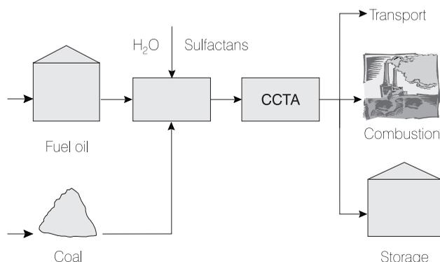
Figure 1. CCTA preparation process
