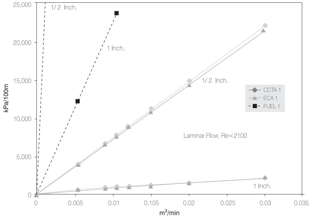
Figure 4a. Pipeline transport simulation for the CCTA mixture, 303 K
