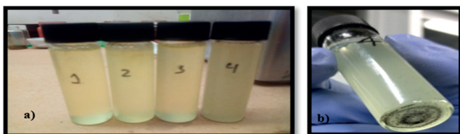
Figure 5. Stability tests performed using ultrasonic bath (GO@Fe 3 O 4 2:1) a) t=0s, b) t=12h
